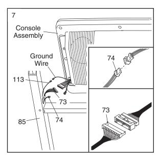
Set the console assembly on the Uprights (85). Make sure that no wires are pinched. Finger tighten a Console Bolt (72) with a Star Washer (67) into the lower hole in each Upright (only one side is shown).
